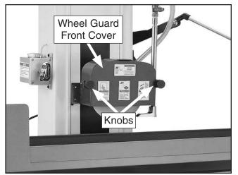
Figure 35. Wheel guard components.
